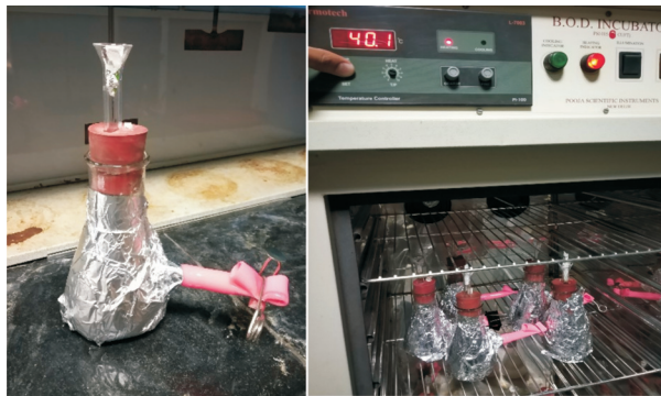
Fig. 5. Acetogenesis batch reactor and incubation
